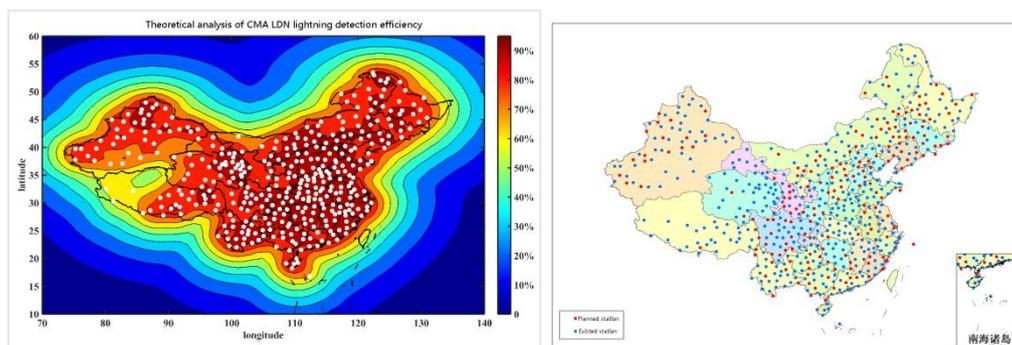
Fig.1 Left is theoretical distribution map of detection efficiency, right is CMA LDN station distribution plan map (blue point is existed station, red point is planned station, total station number is 599) .
