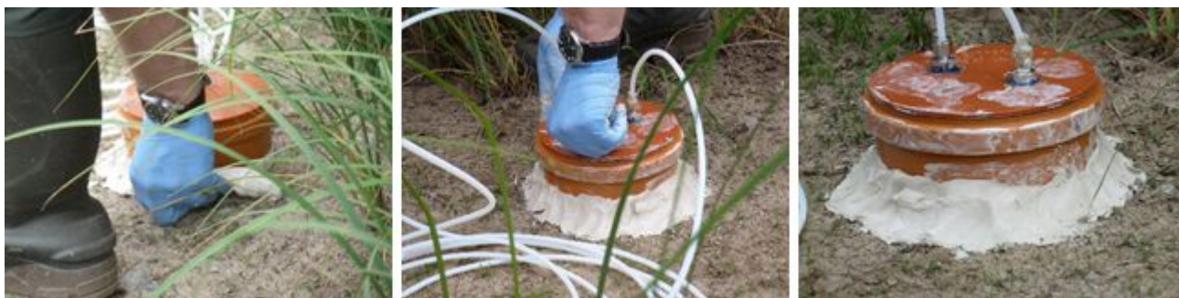
Figure S3: Sealing the chamber with clay.
