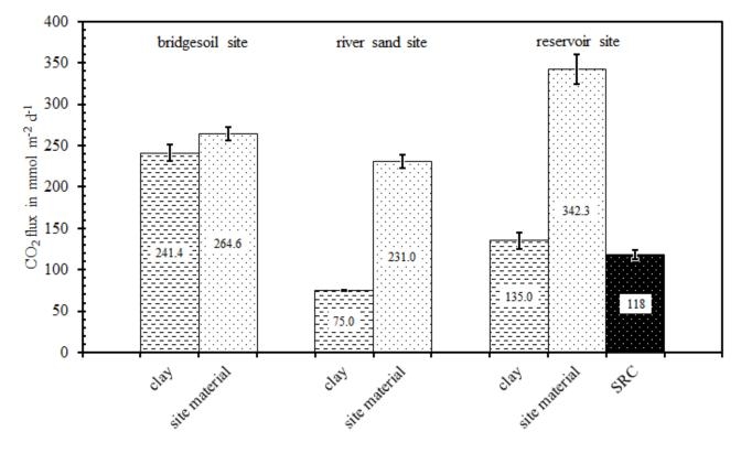
Figure 2: Mean CO<sub>2</sub> fluxes detected in the different sample groups during field experiments (mean  $\pm$  SD, n = 3; reservoir site n = 4). SRC = soil respiration chamber + IR analyser, sealed with clay.
