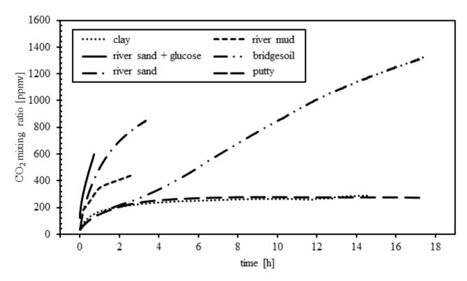
Figure 1: CO<sub>2</sub> concentration during long-term laboratory chamber experiments with different sealing materials.
