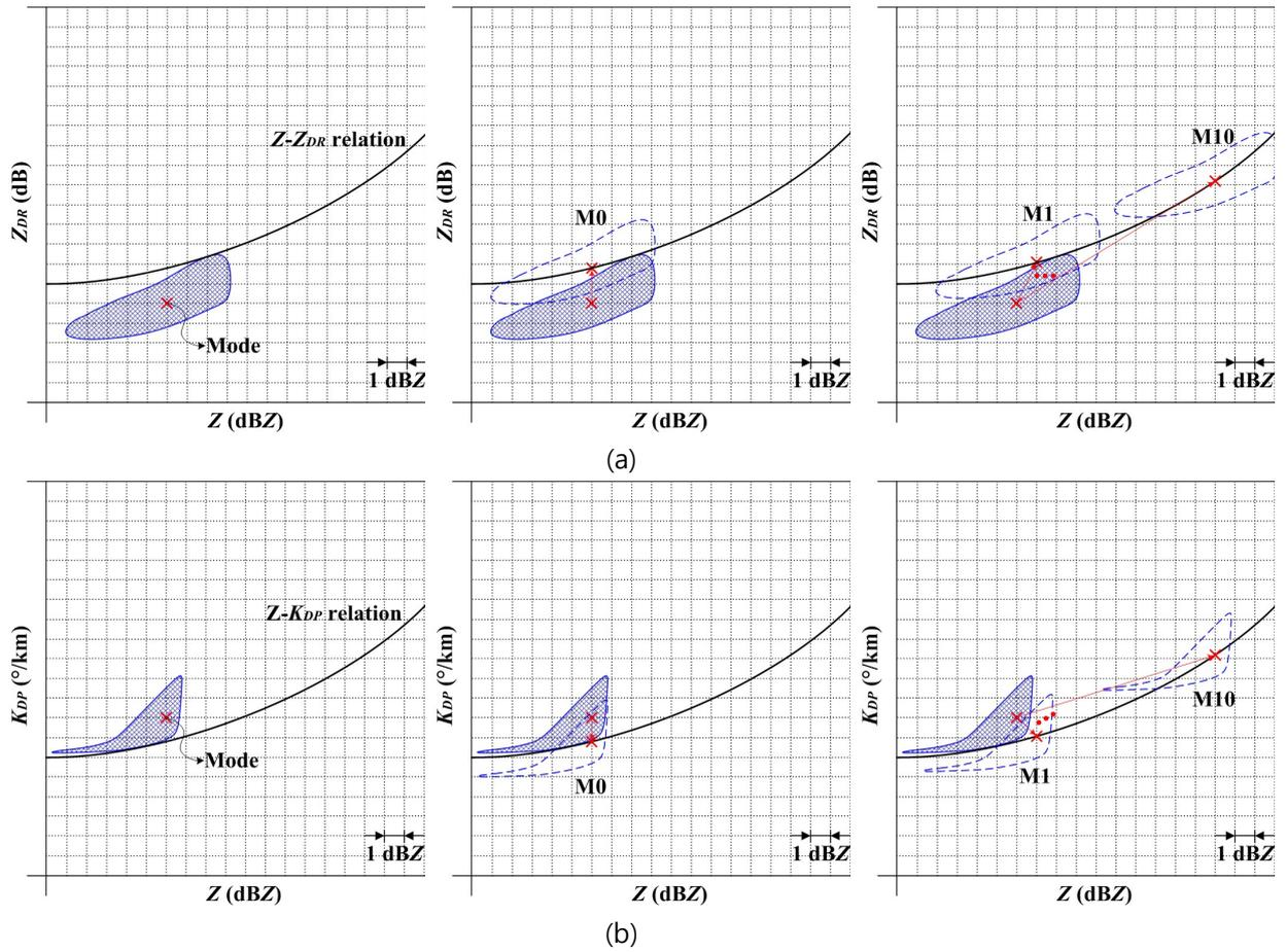
**Figure 3.** Schematic diagram of observed bivariate distribution (left panel) and bivariate distribution shift (middle panel:  $Z$  has no bias, right panel:  $Z$  has bias): (a)  $Z - Z_{DR}$  space and (b)  $Z - K_{DP}$  space
