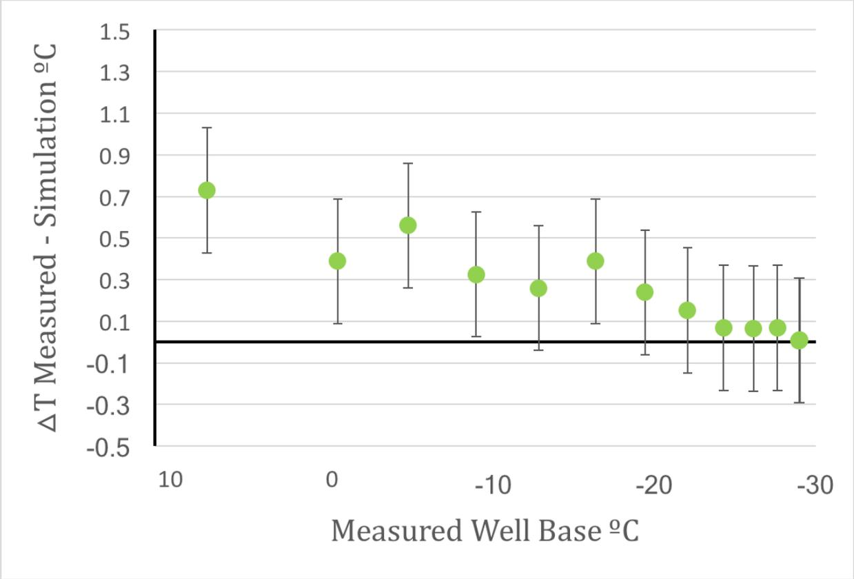
**Figure S1: Difference between measured and simulated temperature of the air pocket in the well base.** The maximum difference between the predicted temperature and the measured temperature over the twelve time steps of the 3276s simulation was 0.6 °C at subzero temperatures. The error bars shown represent the uncertainty of the thermal probe at the well base,  $\pm 0.3$  °C.
