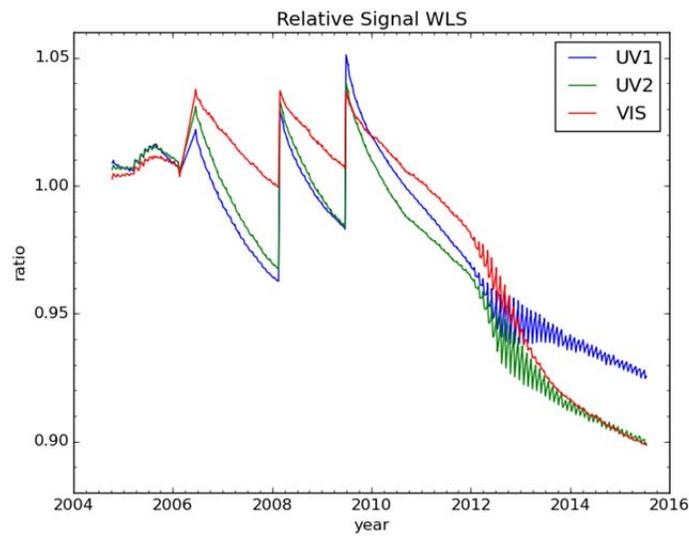
**Figure 7: Signal change of WLS during the mission. Each datapoint shows a measurement divided by a reference measurement from the beginning of the mission. The three abrupt throughput changes in 2006 – 2009 are caused by the long (14 minutes each) WLS duty cycles.**
