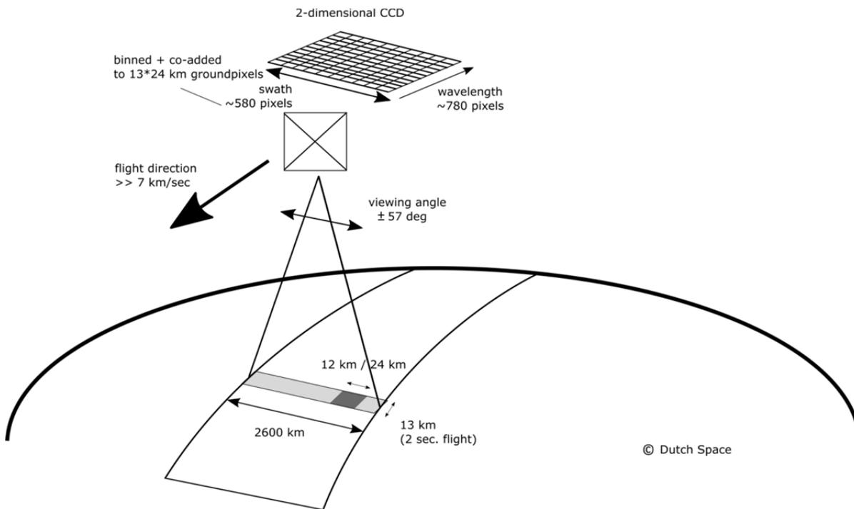
5 **Figure 1: An impression of OMI flying over the earth globe. The spectrum of a ground pixel is projected on the wavelength dimension of the CCD (the columns). The cross-track ground pixels are projected on the swath dimension of the CCD (the rows). The forward speed of 7 km/sec and an exposure time of 2 seconds lead to a ground pixel size of 13 km in the flight direction. The viewing angle of 114 degrees leads to a swath width on the ground of 2600 km.**
