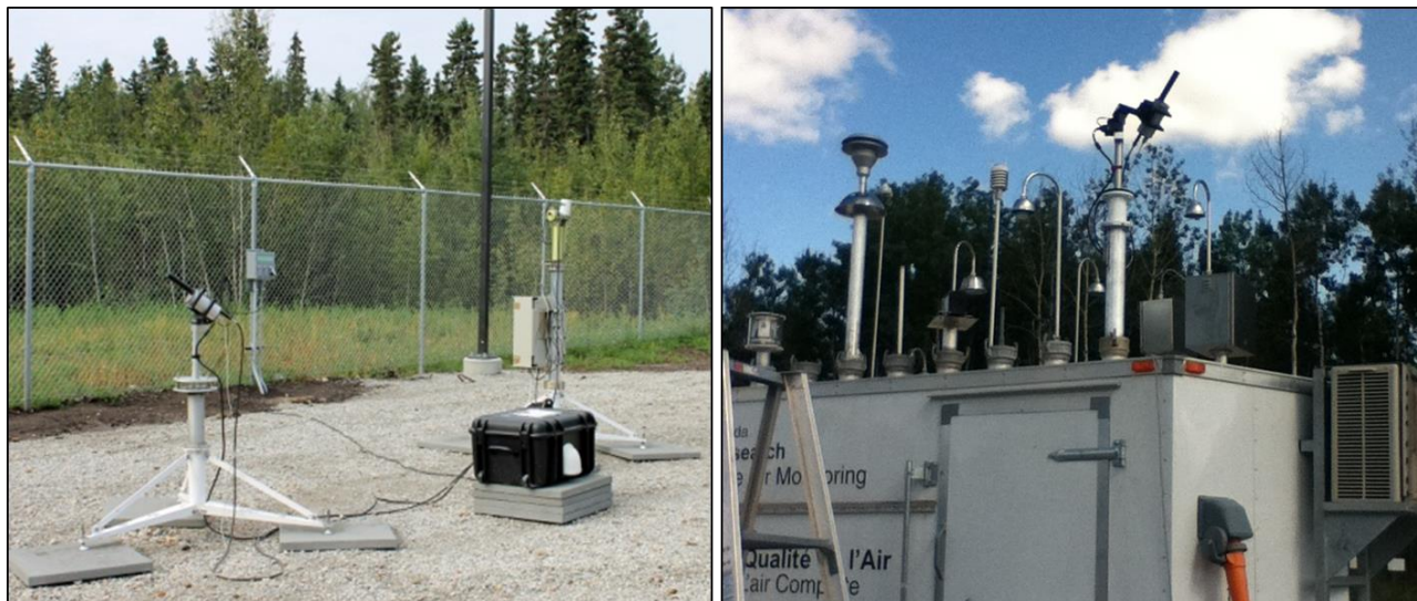
Figure 1. Pandora instruments at Fort McKay in (left) 2013 and (right) 2014-2015. In 2013, the instruments head was installed on a white Brewer tripod and the spectrometer and computer were inside the black box to the right. From 2014, the head was installed on the roof of a trailer with the spectrometer and computer located inside the trailer.
