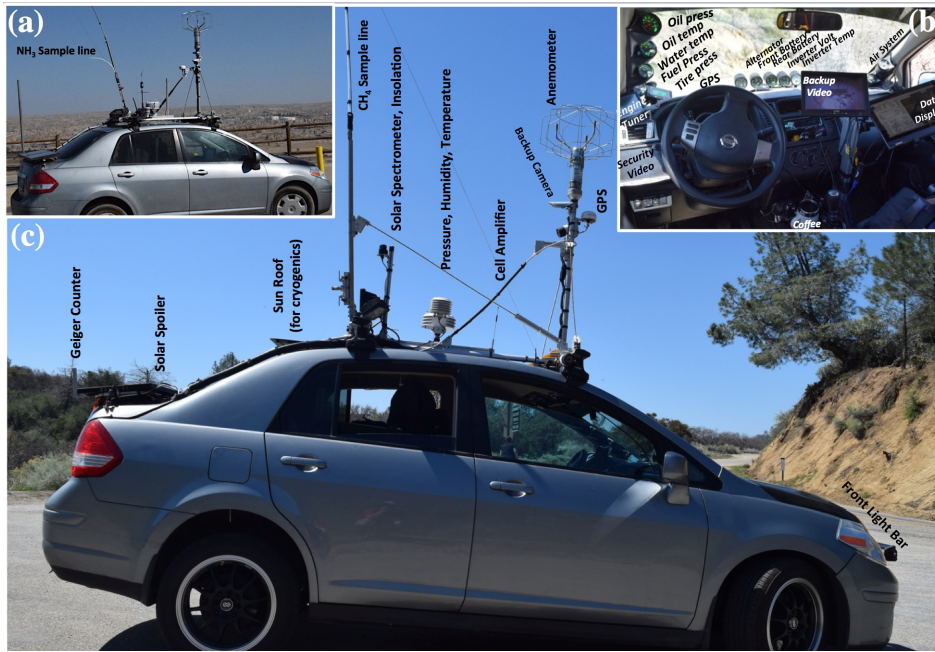
20 Figure S2. (a) AMOG Surveyor in the Transverse Coastal Range (1300 m) – San Joaquin Valley 21 in background. (b) Cockpit view of gauges, security video, rear video, real-time data display. V_A , 22 V_{FB} , V_{RB} , V_I – voltages for alternator, front battery, rear battery, inverter. T_I , T_O , T_W – temperatures 23 for inverter, engine oil, and radiator water. P_T , P_O , P_W , P_S , P_C , P_R – pressures for tires, oil, water 24 suspension, compressor, and regulated air for chemical scrubbers. (c) AMOG Surveyor in Sierra 25 Nevada Mountains, roof package labeled.
