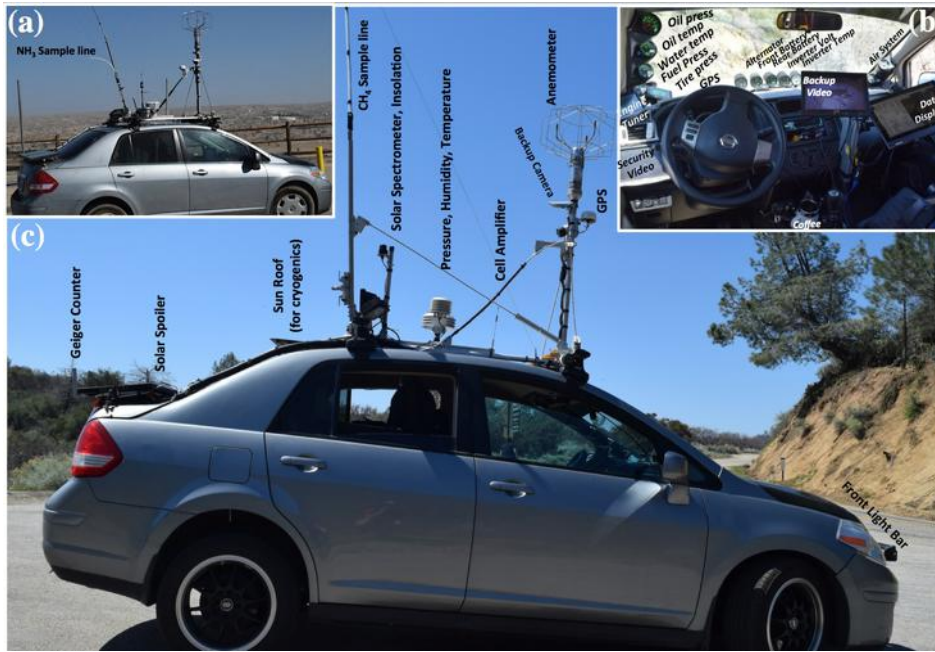
20 Figure S2. (a) AMOG Surveyor in the Transverse Coastal Range (1300 m) – San Joaquin Valley 21 in background. (b) Cockpit view of gauges, security video, rear video, real-time data display. V_A , 22 V_{FB} , V_{RB} , V_I – voltages for alternator, front battery, rear battery, inverter. T_b , T_o , T_w – temperatures 23 for inverter, engine oil, and radiator water. P_T , P_o , P_w , P_s , P_C , P_R – pressures for tires, oil, water 24 suspension, compressor, and regulated air for chemical scrubbers. (c) AMOG Surveyor in Sierra 25 Nevada Mountains, roof package labeled.
