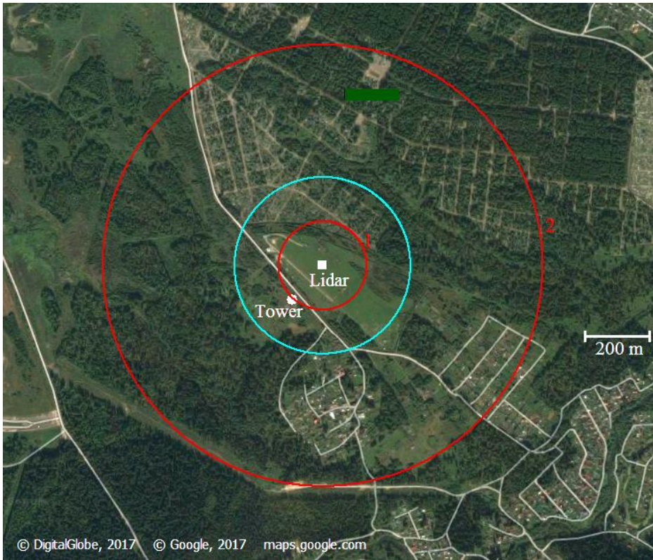
5 Figure 3: Map of the experimental site in 2014 and 2016. The blue circle shows the trajectory of the lidar sensing volume at a height of 43 m during the measurement at the elevation angle \varphi = 9^\circ in 2014. Red circles 1 and 2 shows the trajectories of the lidar sensing volume at heights of, respectively, 100 and 500 m during the measurement at \varphi = 35.3^\circ in 2016. Coordinates of the lidar point were 56^\circ 28' 51.41''\text{N} , 85^\circ 06' 03.22''\text{E} .
