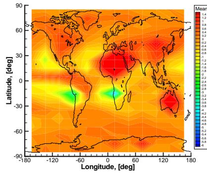
**Figure 8.** Deviation statistics based on original BLB-corrected bending angles:: latitude-longitude map of inversion statistics of COSMIC observations relative to ECWMF profiles without fluctuations, for refractivity at altitude of 0.6 km. Results are shown for COSMIC events and concurrent ECWMF analysis fields from the 1st, 11th, and 21th day of every month of year 2008.
