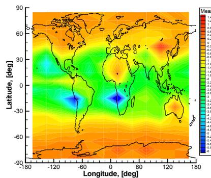
**Figure 3.** Deviation statistics obtained for real RO data: latitude-longitude map of inversion statistics of COSMIC observations relative to ECWMF profiles without fluctuations, for refractivity at altitude of 0.6 km. Results are shown for COSMIC events and concurrent ECWMF analysis fields from the 1st, 11th, and 21th day of every month of year 2008.
