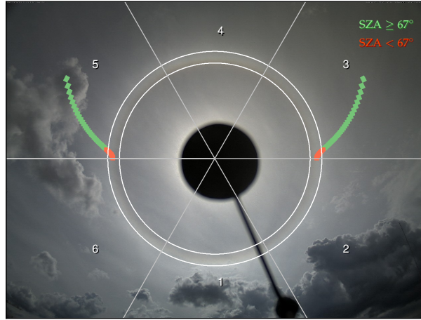
Figure 9. HaloCam image as in Fig. 4b. The red and green squares indicate the minimum scattering angle of the sundogs as a function of the solar zenith angle (SZA). The SZA ranges between 90^\circ and 35^\circ with 1^\circ resolution. The mask used to search for the 22^\circ halo peak is displayed by the two white circles and covers scattering angles between 21.0^\circ and 23.5^\circ . Sundog positions located within this mask might be mis-classified as 22^\circ halo and are marked as red. These positions correspond with SZAs between 90^\circ and 67^\circ . For smaller SZAs (higher solar elevations) the sundogs are located outside the mask and cannot be mis-classified as 22^\circ halo by the algorithm.
