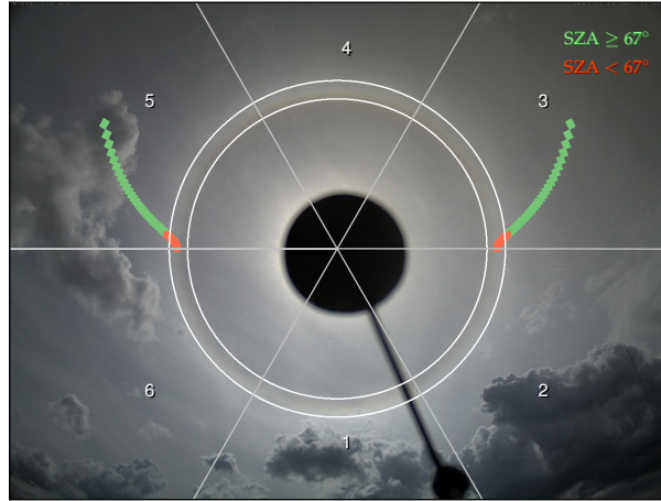
Figure 9. HaloCam image as in Fig. 4b. The red and green squares indicate the minimum scattering angle of the sundogs as a function of the solar zenith angle (SZA). The SZA ranges between 90^\circ and 35^\circ with 1^\circ resolution. The mask used to search for the 22^\circ halo peak is displayed by the two white circles and covers scattering angles between 21.0^\circ and 23.5^\circ . Sundog positions located within this mask might be mis-classified as 22^\circ halo and are marked as red. These positions correspond with SZAs between 90^\circ and 67^\circ . For smaller SZAs (higher solar elevations) the sundogs are located outside the mask and cannot be mis-classified as 22^\circ halo by the algorithm.
