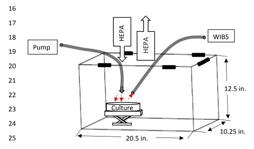
26 <u>Figure S1.</u> Schematic diagram of home-built chamber for the aerosolization of fungal spores.
