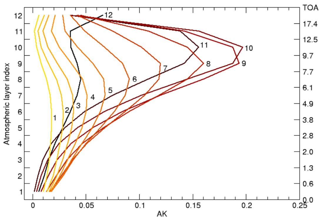
**Figure 1.** A typical averaging kernels for GOSAT-TIR daytime measurements over land. The colour coding is such that dark colours correspond to the averaging kernels at high altitudes and the bright colours to low altitudes. The numbers next to the curves refer to the corresponding atmospheric layer index as is indicated on the left side of the graph.
