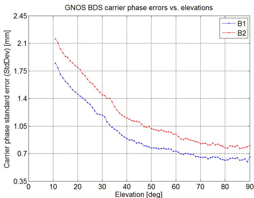
**Figure 3.** Statistics of FY-3C GNOS BDS carrier phase standard deviations (blue, B1 signal carrier phase; red, B2 signal carrier phase) as function of elevation angle, calculated by using positioning channel measurements.
