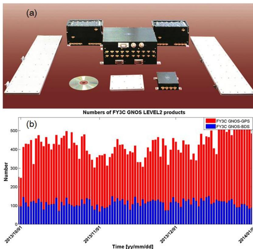
**Figure 1.** Components of the GNOS instrument (setting/rising occultation antenna and RF unit, left/right; navigation antenna and RF unit, middle in front; tracking and data processing unit, middle in back) (a), and illustration of the daily number of high-quality FY-3C GNOS GPS and BDS RO events for October-December 2013 as used in this study (b).
