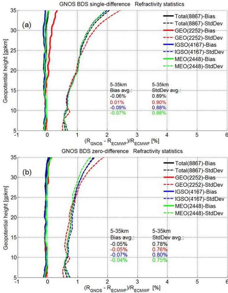
**Figure 8.** Mean difference (Bias) and standard deviation (StdDev) statistics of the GNOS refractivity profiles retrieved by using excess phases from the single-difference processing (a) and the zero-difference processing (b), respectively, with the co-located ECMWF refractivity profiles used as reference. Same layout as Figure 6; see that caption for further description.
