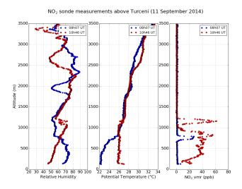
Figure 6. Lower parts of two  $NO_2$  balloon-borne sonde measurements in Turceni on 11 September 2014. The left panel presents the profiles of relative humidity during the two soundings, the middle panel presents the potential temperature profiles, and the right panel presents the  $NO_2$  profiles.
