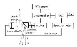
Figure 1. Schematic diagram of the SWING instrument.
