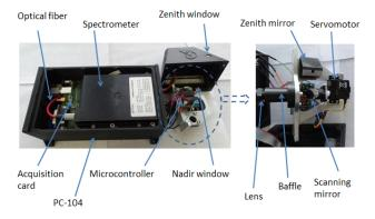
Figure 2. The SWING instrument. Its dimensions are 27x12x8 cm<sup>3</sup> and its weight is 920 g.
