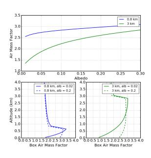
Figure 10. Calculated nadir air mass factors in the AROMAT conditions, respectively from 800 m altitude and 3 km altitude.
