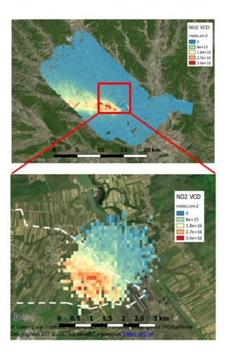
Figure 11. SWING, AirMAP, and Mobile DOAS measurements of  $NO_2$  in Turceni on 11 September 2014. The upper panel shows the AirMAP and Mobile-DOAS measurements (see text) while the lower panel shows the SWING measurements superimposed on the trace of the plume seen by AirMAP (dashed white line).
