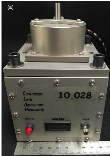
Figure 1: (a) Photograph of CLAP, and (b) cross-sectional view of flow and optical paths in upper section and three-dimensional view of CLAP internal configuration in lower section. Scale on ruler in left image is in millimeters. An annotated version of (b) is included in the Supplement (Fig. S1).
