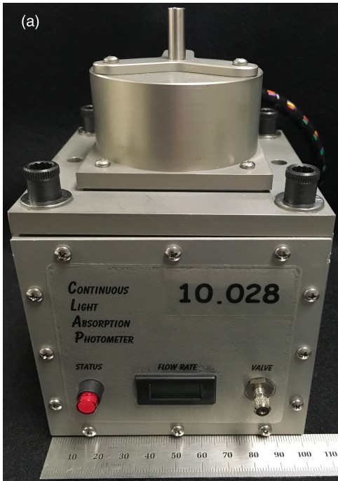
5 Figure 1: (a) Photograph of CLAP, and (b) cross-sectional view of flow and optical paths in upper section and three-dimensional view of CLAP internal configuration in lower section. Scale on ruler in left image is in millimeters. An annotated version of (b) is included in the Supplement (Fig. S1).
