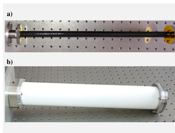
Figure 2. Home made multipass cell in the open-cell configuration (a) and in the closed-cell configuration (b).
