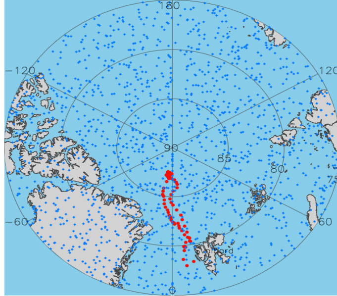
Figure 1: Radiosonde soundings track (red dot) during ASCOS field campaign from 3 August to 7 September 2008, and the COSMIC RO (e.g., UCAR) soundings distribution (blue diamond) during the same time period over 75°N-90°N.
