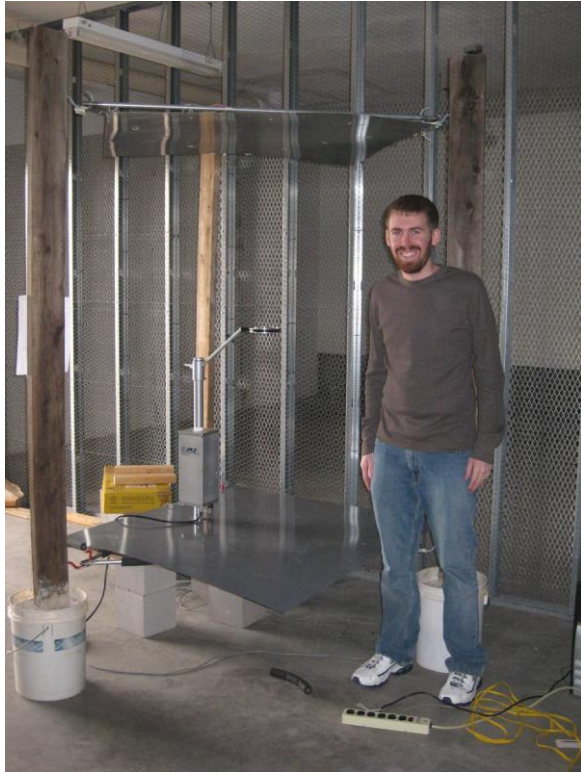
Figure 2 – Picture taken during indoor testing showing a hotplate's precipitation sensor positioned between top and bottom painted-steel sheets.
