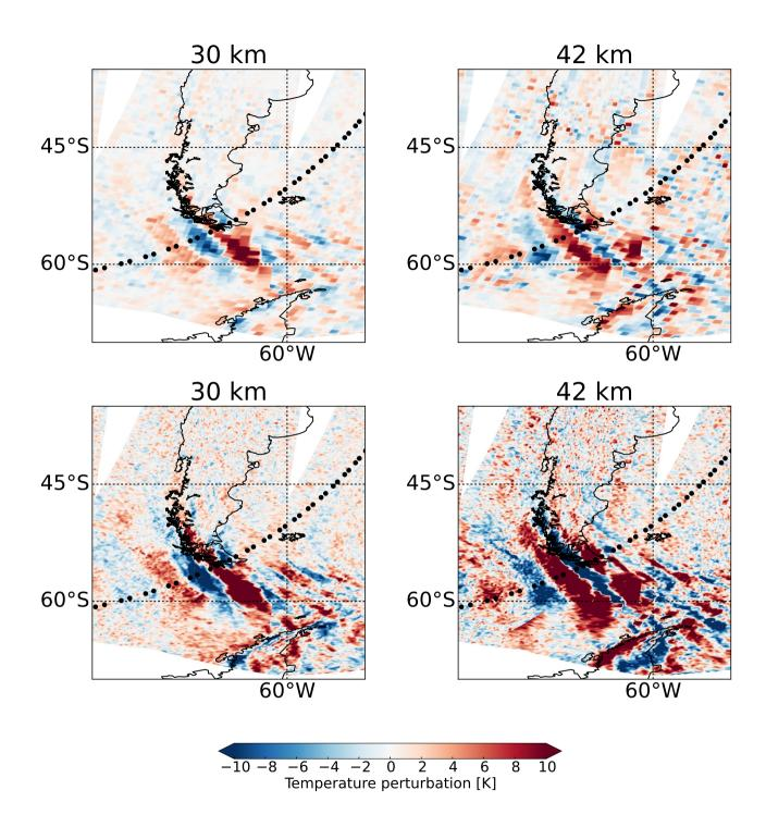
**Figure 4.** Temperature perturbations from AIRS retrievals on 29 September 2006 about 3 UTC at 30 km (left) and 42 km (right) for a mountain wave event near Tierra del Fuego. – Top: AIRS operational retrieval. Bottom: AIRS high-resolution retrieval. Black circles indicate the locations of HIRDLS profiles.
