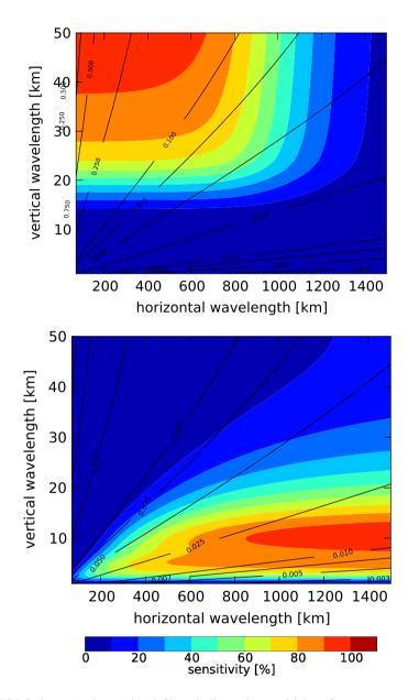
**Figure 3.** AIRS (top) and HIRDLS (bottom) observational filters indicate the sensitivity of temperature variances to gravity waves with different horizontal and vertical wavelengths. The black lines show a momentum flux factor (see text for details).
