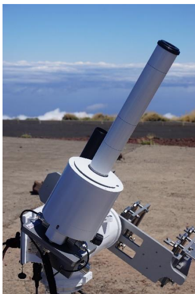
Figure 3 The BTS2048-UV-S-WP modified for direct solar measurements mounted on a solar tracker at the Izaña observatory in Tenerife.
