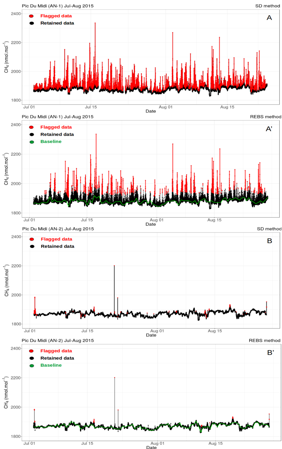
590 Figure 3: AN-1 CH 4 measurement at T55 building for A and A', and AN-2 TDF building for B and B'. Black data points are the retained measurements, red points represent the flagged using SD method for A and B, and REBS method for A' and B'
