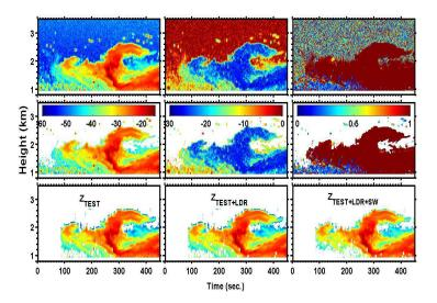
Fig. 2. Figure AR2: TEST performance in filtering biota echoes that are co-present with low clouds.
