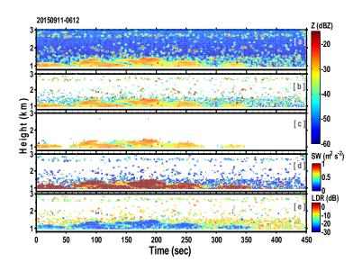
**Fig. 1.** Figure AR1: HTI plot of cloud radar measured (a) Reflectivity (Z), (b) noise removed Z, (c) TEST filtered Z, (d) Spectral Width (SW), and (e) LDR at 0612 UT on 11 Sep 2015.
