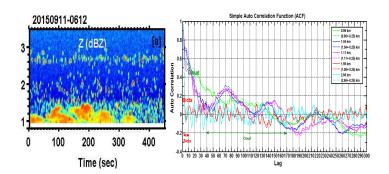
**Fig. 4.** Figure AR9: Shallow cumulus cloud present with biota (HTI plot) and (right panel) is AFC based 0-300 lag correlation for cloud and biota.
