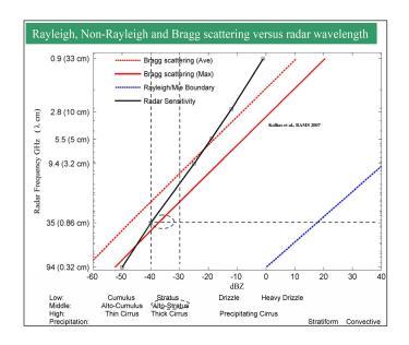
Fig. 2. Figure AR7: Atmospheric radar echo scattering Vs radar wavelengths (taken from Kollias et al., BAMS 2007).
