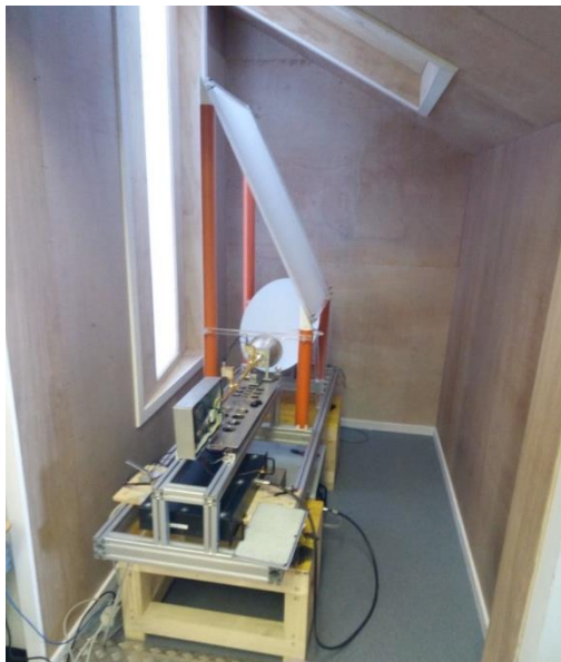
Figure 1: (a), a picture of the instrument installed at the THAAO, Thule Air Base, Greenland where the two ecofoam windows can be seen. (b), a scheme of the instrument VESPA-22.
