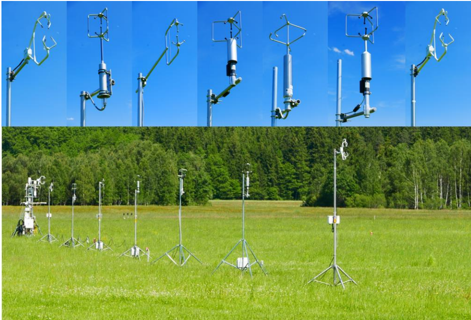
Figure 2: The bottom part of this figure shows a photograph of the field intercomparison experiment; the micrometeorological installations of the TERENO/ICOS site DE-Fen can be seen in the background (left). On top, close-up pictures of all seven sonic anemometers are shown; they are presented from left to right in the same order as they are listed in Table 1.
