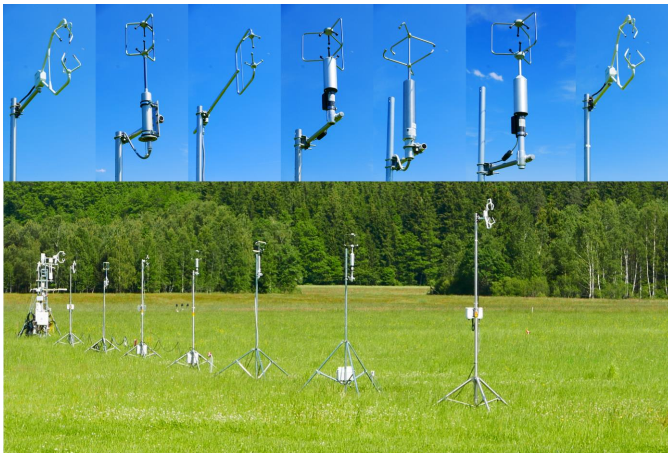
Figure 2: The bottom part of this figure shows a photograph of the field intercomparison experiment; the micrometeorological installations of the TERENO/ICOS site DE-Fen can be seen in the background (left). On top, close-up pictures of all seven sonic anemometers are shown.
