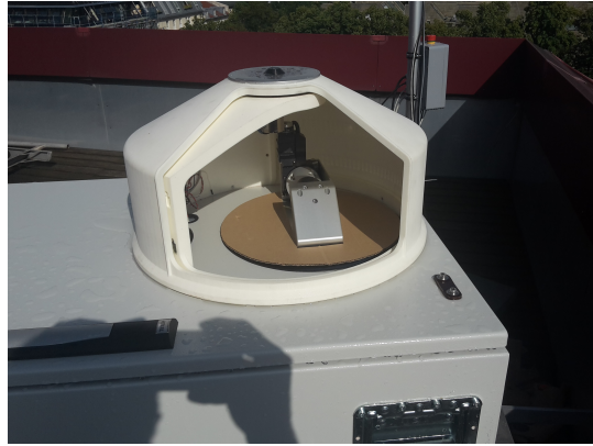
Figure 13. (a) Image of flooded stair house. The water was blown into the tilted window. (b) Image of the open enclosure after the storm. As can be seen, no water was able to penetrate the cover.
