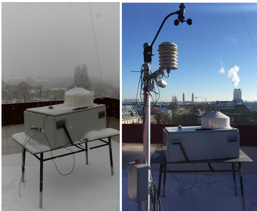
Figure 14. (a) During 2016 winter, inches of snow fall on the enclosure with the spectrometer located inside. (b) The system is taking measurements in cold winter below 0°C.
