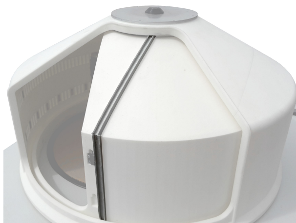
Figure 5. The image shows the gasket that were installed to seal the gap between the two caps. It prevents water from being blown into the cover by strong winds.
