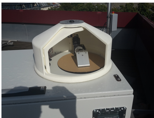
Figure 13. (a) Image of flooded stair house. The water was blown into the tilted window. (b) Image of the open enclosure after the storm. As can be seen, no water was able to penetrate the cover.
