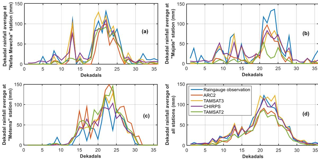
**5 Figure 7: Comparison of the satellite products with the rain gauge observations at wider elevation range based on dekadal average for 2000-2015 a) at “Nefas Mewucha” station with an elevation of 3098 m a.s.l, b) at “Majate” stations with an elevations of 2000 m a.s.l, c) at “Metema” stations with an elevation of 790 m a.s.l, and d) at dekadal rainfall average from all rain gauge stations. The x-axis represents the 36 dekadals of year.**
