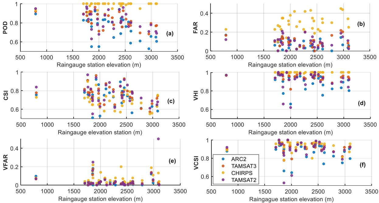
5 **Figure 5: Categorical and volumetric validations of satellite rainfall products at different elevation values: (a) Probability of Detection (POD), (b) False Alarm Ratio (FAR), (c) Critical Success Index (CSI), (d) Volumetric Hit Index (VHI), (e) Volumetric False Alarm Ratio (VFAR), and (f) Volumetric Critical Success Index (VCSI).**
