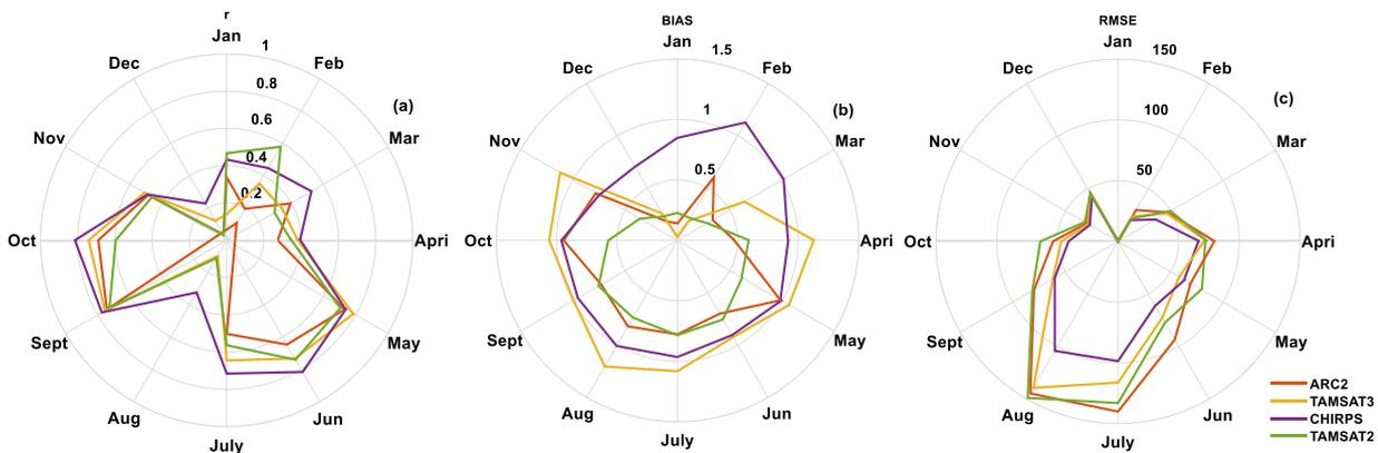
Figure 10: Statistical validation of the satellite products at each twelve months of the UBN basin for 2000-2015. (a) Pearson correlation coefficient ( $r$ ), (b) Bias ratio, and (c) Root mean square error (RMSE).
