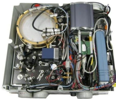
Figure 1: (a) Schematic of the instrument with the key optical and hardware elements. (b,c) Photograph of the QCLAS with the top cover removed and in the final layout. The overall weight is 10 kg and it operates on 12V DC.
