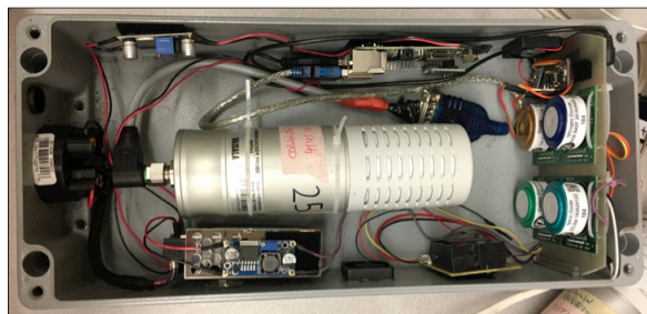
Figure 2. Current BEACO 2 N node design.
