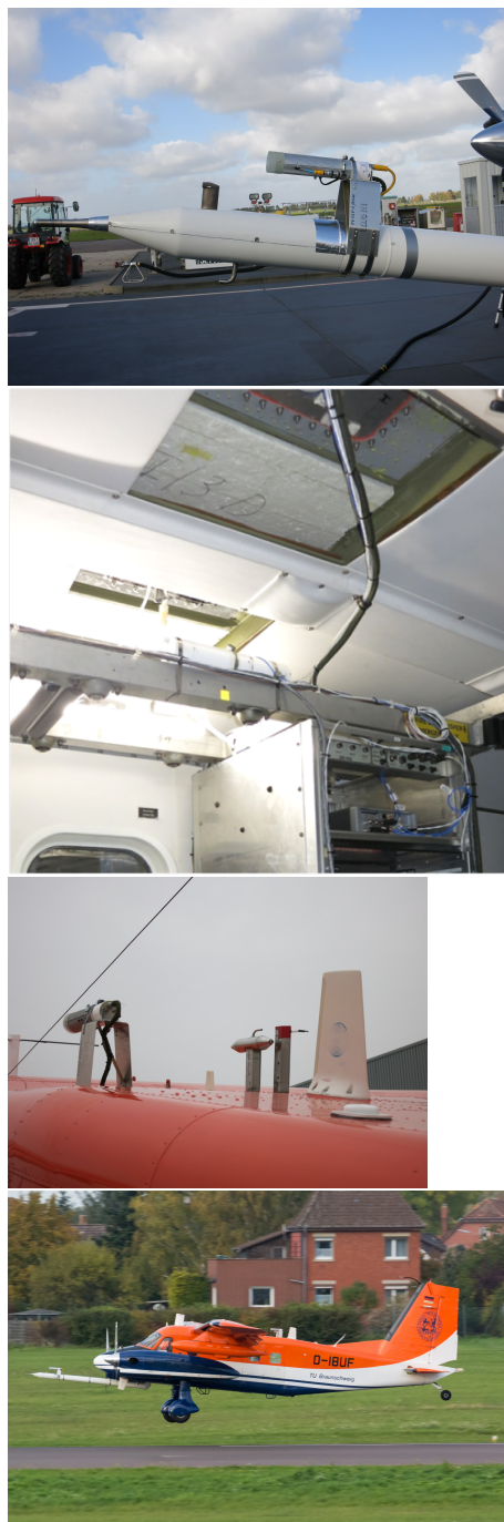
Figure 1. The three LICOR sensors integrated into the Do128 during a humidity intercomparison flight: a) LI7500A on the nose boom (Li1), b) LI7200 in the cabin with an inlet near the LICOR sensor on the roof (Li2), c) LI7500 on the roof (Li3), and d) the Do128 equipped with additional sensors during the flight (last photo courtesy of Uwe Bethke).
