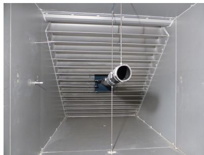
Figure 22. Ice particle conveyance pipe inside the settling chamber of the Braunschweig Icing Wind Tunnel
