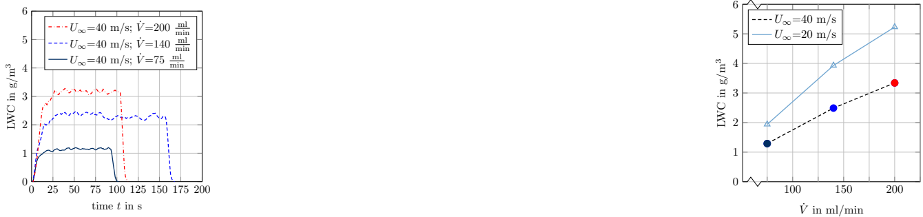
Figure 29. Liquid water content calibration based on IKP measurements. Left: LWC history. Right: LWC depending on supplied water flow-rate.
