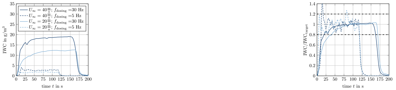
Figure 31. IWC time history based on IKP measurements. Left: IWC history. Right: Normalized IWC history.
