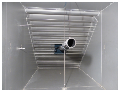
Figure 23. Ice particle conveyance pipe inside the settling chamber of the Braunschweig Icing Wind Tunnel
