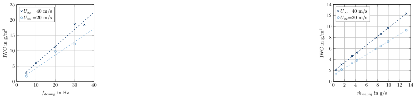
Figure 32. Ice water content depending on dosing frequency f_{\text{dosing}} and injected ice particle flow \dot{m}_{\text{ice,inj}}
