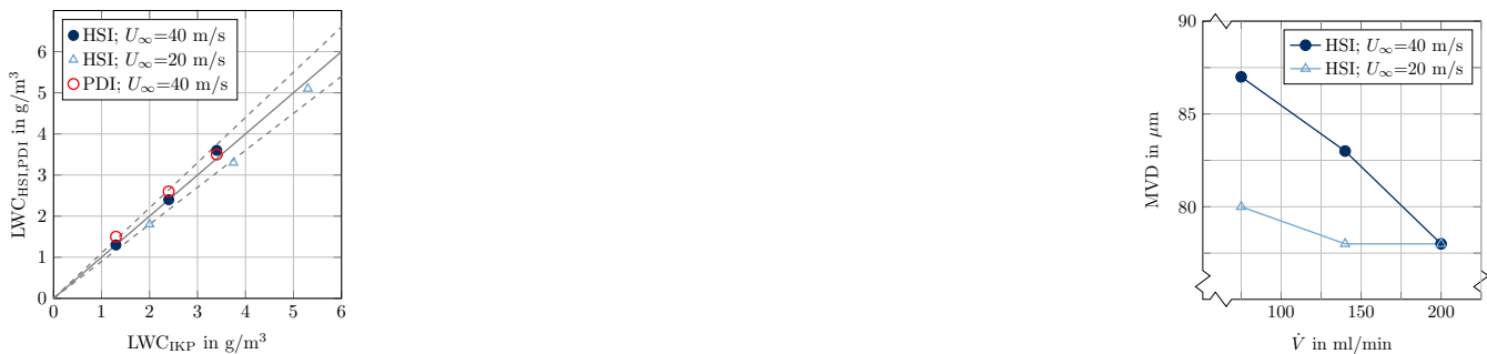
Figure 30. Comparison of HSI, PDI and IKP measurements for supercooled droplet conditions. Left: Optical array probes vs. IKP. Right: MVD vs. LWC.
