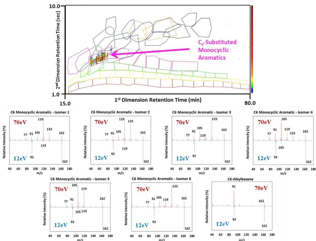
**Figure 2.** A contour plot (chromatogram) displaying C<sub>6</sub>-substituted monocyclic aromatics identified by the CLIC expression. All C<sub>6</sub>-substituted monocyclic aromatics are located within the pink polygon displayed. 70eV (red peaks) and 12eV (blue peaks) mass spectra corresponding to the peaks identified by the CLIC expressions in the SIC is shown for 6 different C<sub>6</sub>-substituted monocyclic aromatics isomers.
