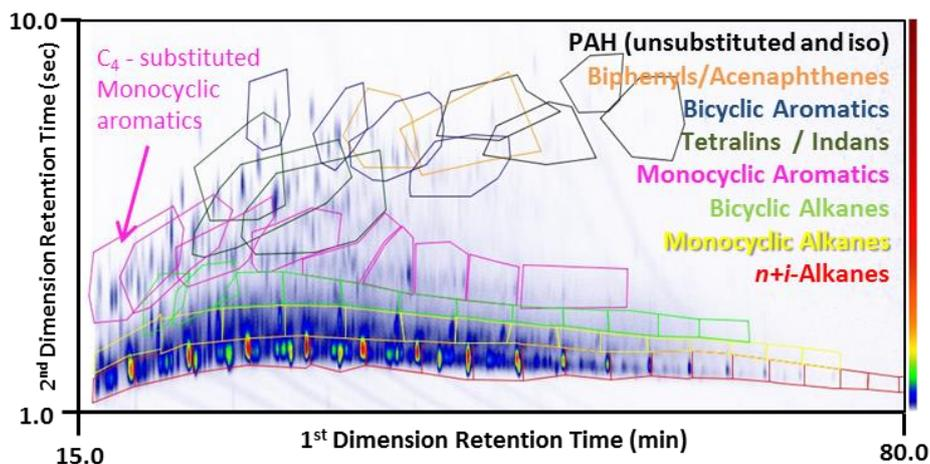
**Figure 1.** A contour plot (chromatogram) of diesel fuel separation. Peak height (intensity) increases with warmth (blue to red) of the colour scale. Each region fenced by a coloured polygon marks out the 2-dimensional chromatogram space in which are found isomers of a particular compound type having a particular carbon number (*e.g.* C<sub>4</sub>-substituted monocyclic aromatics).
