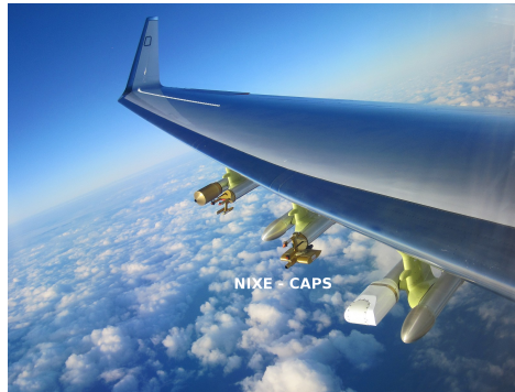
Figure 7. NIXE underwing mounting at HALO (photo: A. Afchine).
