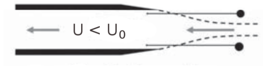
Figure 2. Sub-isokinetic sampling of ice particles by a nearly virtual inlet, where the velocity U inside of the inlet tube is much smaller than the flow speed U_0 . The dashed lines denote the region of the free stream from where the gas streamlines enter the inlet; the black dots illustrate large particles that do not follow the gas streamlines, particle tracks are indicated by thin solid lines (adapted from Krämer et al., 2013).
