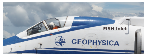
Figure 5. Side mounted FISH-inlet at Geophysica (photo: A. Afchine).
