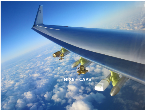
Figure 7. NIXE underwing mounting at HALO (photo: A. Afchine).
