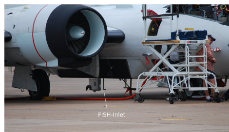
Figure 6. Bottom mounted FISH-inlet at WB-57 (photo: A. Afchine).
