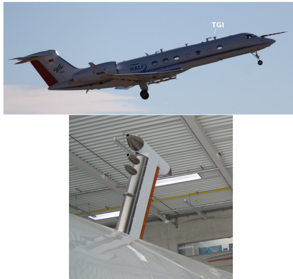
Figure 4. Roof mounted FISH, HAI, Waran inlet at HALO (photos: top A. Fix, bottom A. Afchine).
