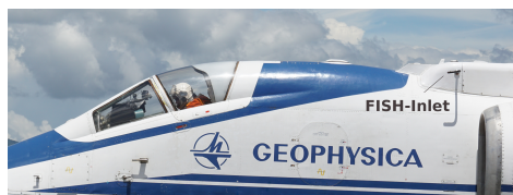
Figure 4. Side mounted FISH-inlet at Geophysica (photo: A. Afchine).
