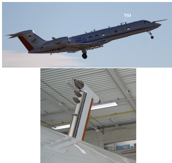
Figure 3. Roof mounted FISH, HAI, Waran inlet at HALO (photos: top A. Fix, bottom A. Afchine).
