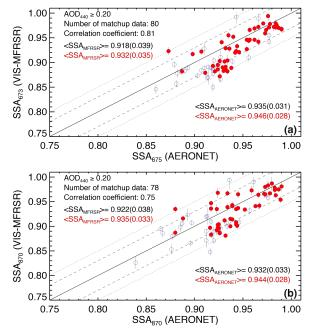
Figure 4. Comparison between SSA at 675 and 870 nm retrieved from AERONET almucantar retrievals and SSA at 673 and 870 nm retrieved from MFRSR DD retrievals.
