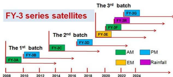
Figure 1. Timeline of FY-3 series satellites. The FY-3 series satellites are the Chinese second generation polar-orbiting meteorological satellites including AM, PM, EM and Rainfall types of satellites, which have been/will be launched in three batches. (Source: Sun et al., 2017)
