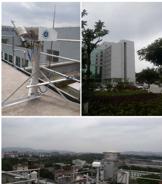
5 Figure 1: The tracker and entrance optics of the Phaethon MAX-DOAS system (upper-left) installed on the roof of the Institute of Geochemistry, Chinese Academy of Sciences, in Guangzhou (upper-right) and an overview of the surrounding area towards West (bottom).
