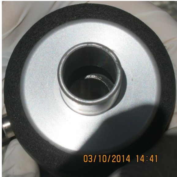
Figure 5: PM 10 pre-impactor plate from the CEM inlet (Line A, Fig. 4) during a routine cleaning after a high wind event.
