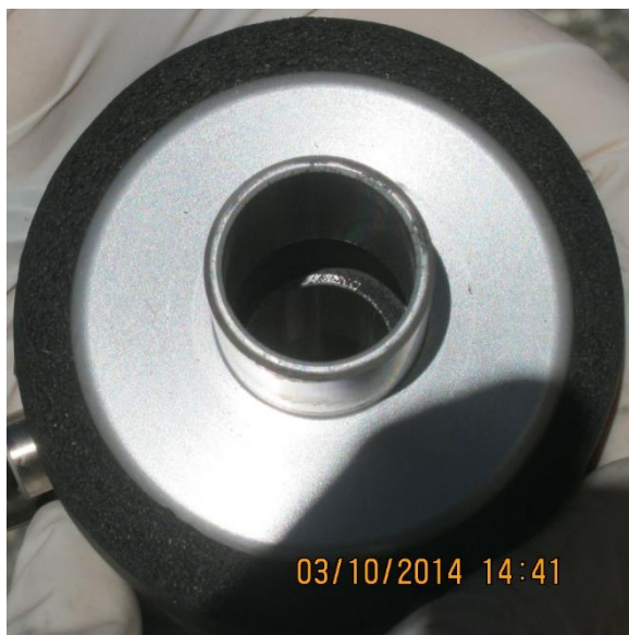
5 Figure 6: Condensation water trap during a cleaning on October 3, 2014. Black powder was visible in the condensation water trap. The black around the outside of the trap is insulating foam.
